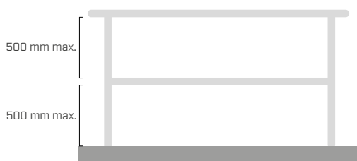
with curb greater than 150 mm
