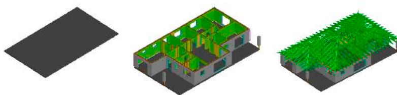
Figure 2. Assembly process of an object with a truss roof.
