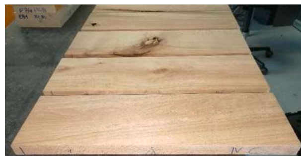
Fig. 4. Examples of beech wood boards containing wood defects detected with NIR spectroscopy.
