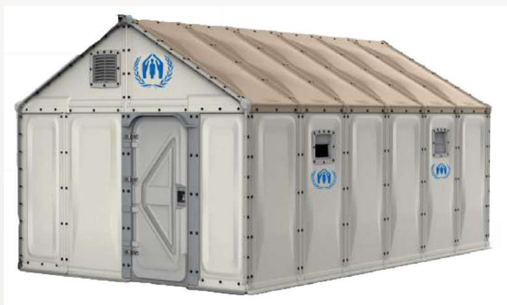
Refuge Housing Unit: 3 years durability; steel frame, polyolefin foam panels, UV stabilized polymer plastic (doors and windows), woven high-density polyethylene fibers (floor)
