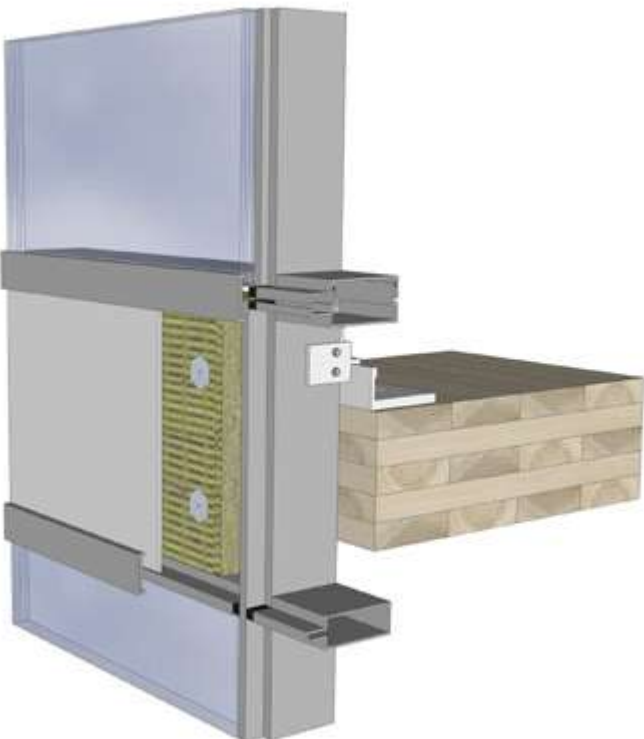
Conventional stick-built or unitized glass and metal curtainwalls offer highly glazed façade options. No different than how they are installed on concrete and steel building structures, glazed curtainwalls provide relatively rapid enclosure to aid in moisture management. Interior finishing requirements are minimal but high window-to-wall ratios should be avoided to conserve energy and enhance thermal comfort. (RDH Building Science Inc.)
