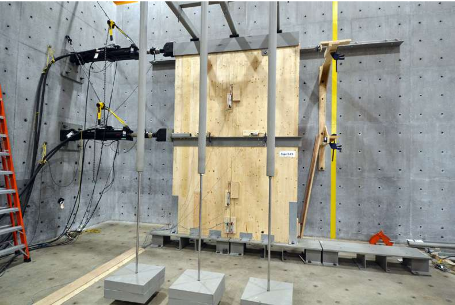
CLT shear wall testing. At the University of Northern British Columbia (UNBC), the testing of connections to CLT panels acting as shear walls has advanced their application in multi-storey buildings. (Fast and Epp)
