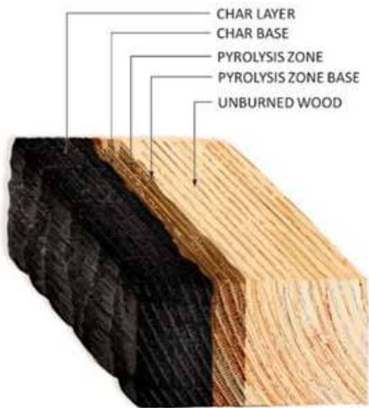
Mass timber is a combustible material that provides impressive fire safety. During fires, exposed mass timber chars on the outside, which forms an insulating layer protecting interior wood from damage. Additionally, when the code requires mass timber to be protected with gypsum wall board, fire testing indicates it can deliver much higher than required fire ratings.
