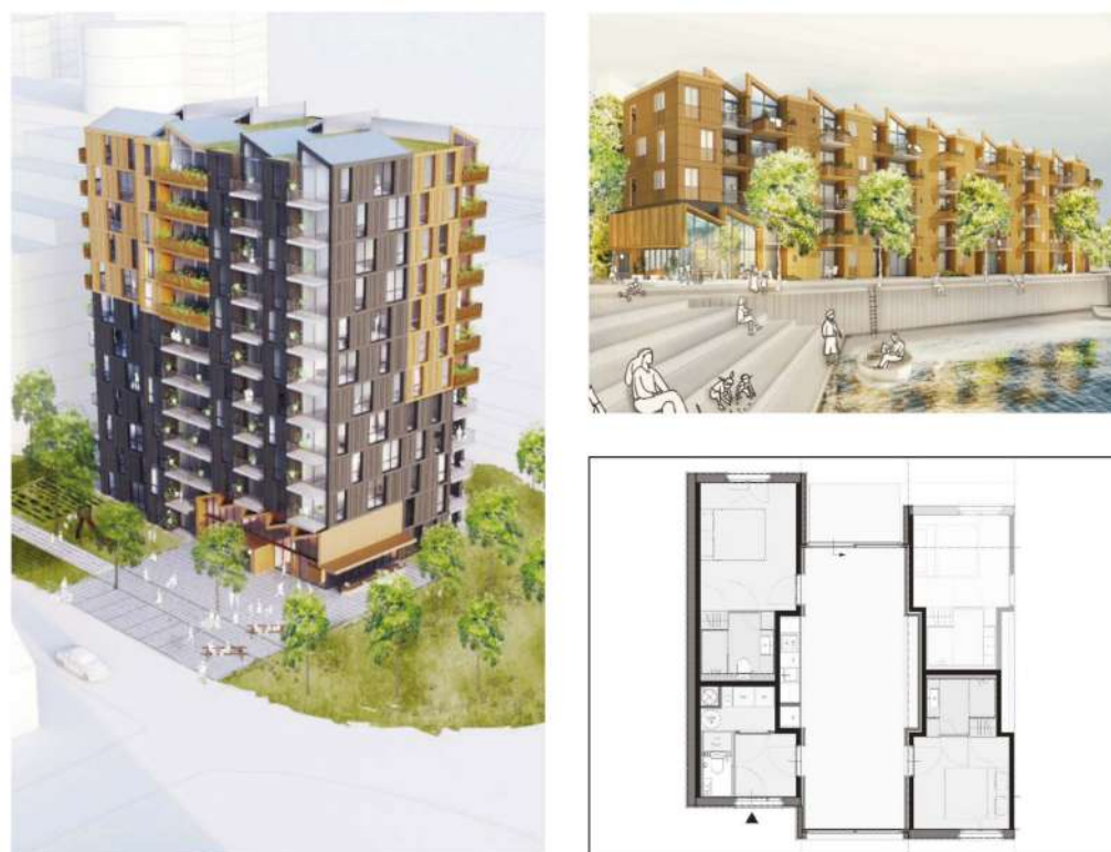
Figure 6. Left, MOOS as multi-storey apartment building up to 70 m height. Right above, a multi-storey building without a lift. Right below, three different modules of MOOS. Source: In the Middle of Our Street.
