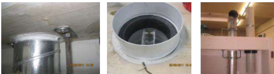
Figure 91: Rigid fastening of the ventilation pipe in the wood floor (left), fire protection closure based on intumescent materials with closing element FLI-VE (center), installation in sample body (right)
