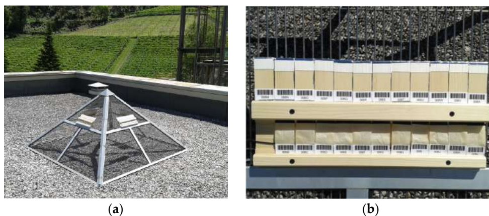
Figure 1. Experimental stand (a) and set of ultra-thin and thick wood samples (b) exposed to natural weathering in San Michele All'Adige (Italy).
