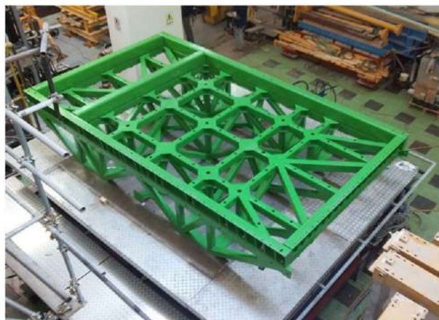
FIGURE 17 Extension and intermediate structure on the shaking table [Colour figure can be viewed at wileyonlinelibrary.com ]
