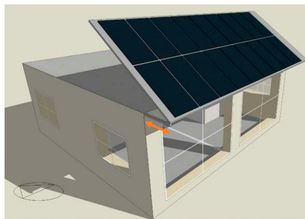
Figure 7. An example of the shading of the southern facade of the modular house with a sliding sun shade element in the form of PV panels on 15 March at 11:00.
