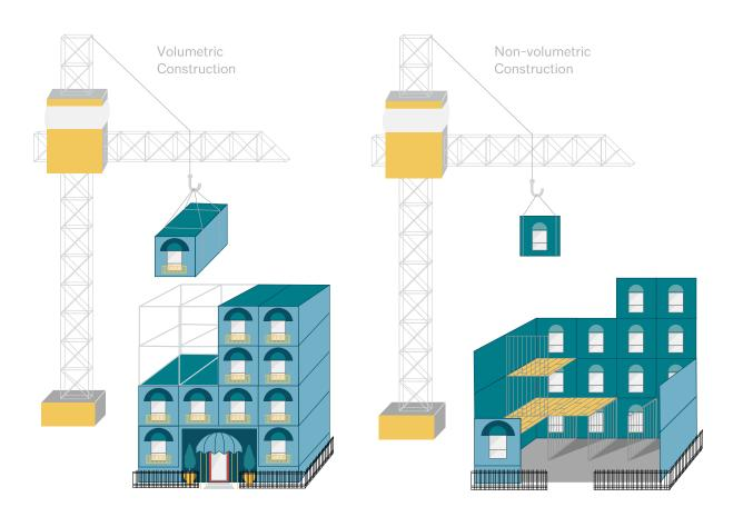
FIGURE 1: VOLUMETRIC VS. NON-VOLUMETRIC CONSTRUCTION
