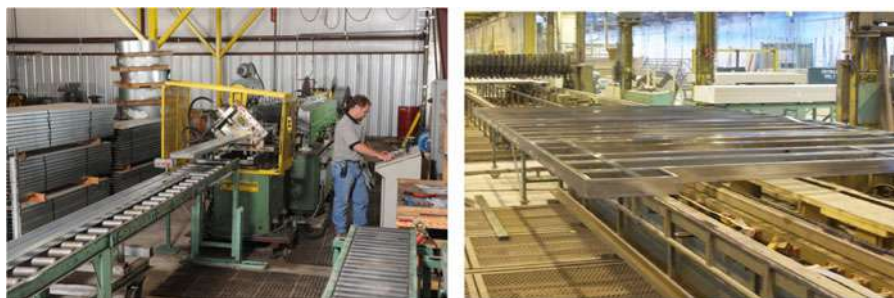
Figure 5. Cold-formed steel wall manufacturing. (Image sources: Deluxe Building Systems)
