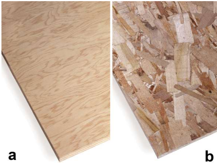
Figure 1.18 Wood-based panels: (a) plywood (photo APA wood), (b) OSB (photo APA Wood).
