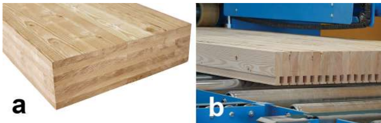
Figure 1.17 Mass timber panels: (a) Cross-laminated timber (Photo APA Wood); (b) Dowel-laminated timber panels (Photo StructureCraft).
