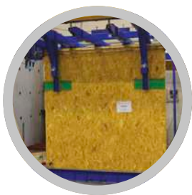
Frame wall during testing
