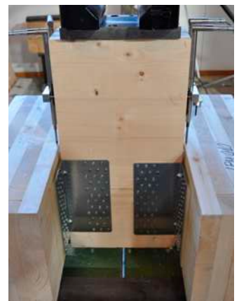
Test samples: 5-layer CLT panels TITAN angle brackets with full fastening TTF200 - TTN240 - TTS240 - TTV240 XYLOFON 35 resilient profile
