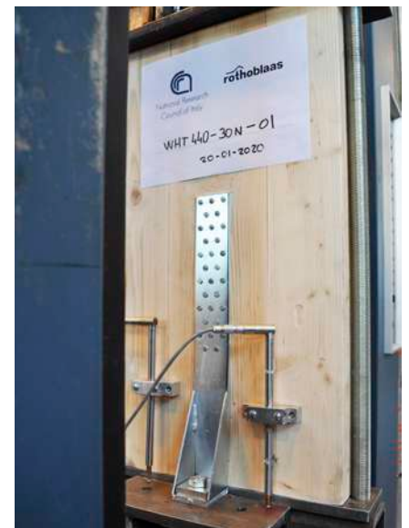
Experimental campaign on CLT panels (C24) (CNR-IBE San Michele All'Adige, 2020).
